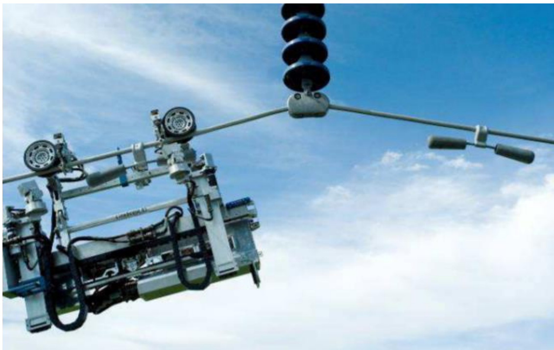
10. ábra LineScout robot a sodronyon [10]
