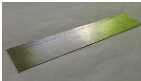
Fig. 4. Sn-Sn solder alloy plate after rolling.
