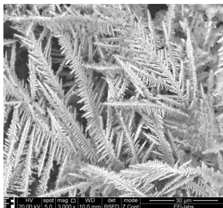
Fig. 1. SEM picture from Sn dendrites.
