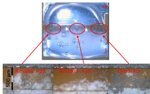
Fig. 9. White colored residue and dendrites were formed in 10mM NaCl solution during WD test in case of galvanic Sn.
