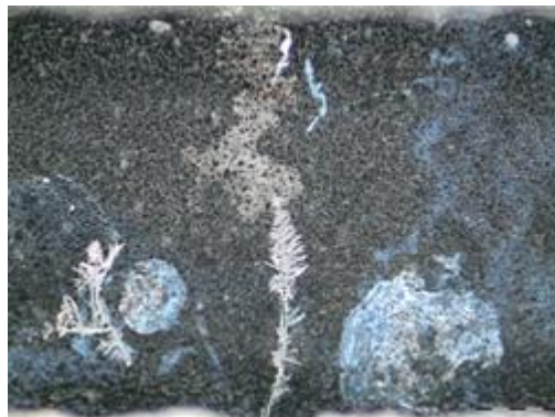
Fig. 6. Dendrites and blue colored residues were formed in 0.1 mM NaCl solution during WD test in case of Sn sample.
