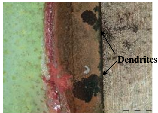
Fig. 10. Dendrites formed in 500mM NaCl TEL during WD test in case of immersion silver.
