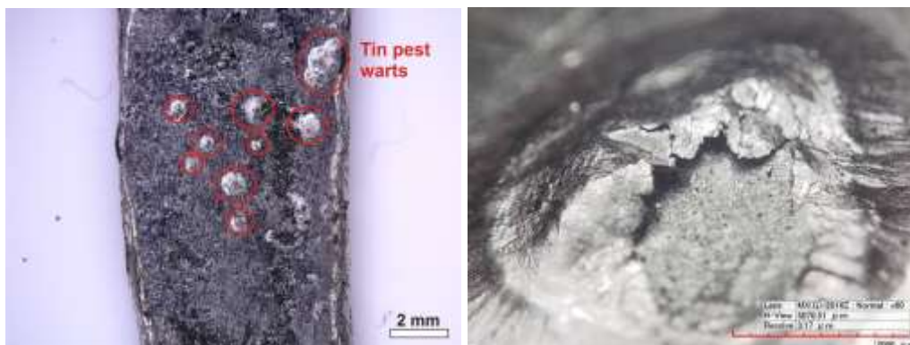
Fig. 1. \beta \rightarrow \alpha transition: a ) \alpha -Sn warts on the surface of Sn object; b) blistering of \alpha -Sn.
