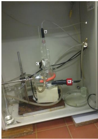
Fig. 1. The electroanalytical measuring platform for LSV test (W-working electrode, C –counter electrode, R-reference electrode).
